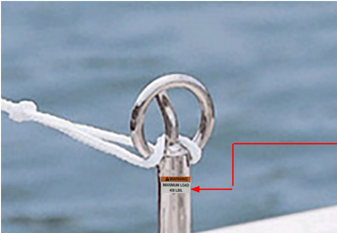
TYPICAL WATER SPORTS OUTBOARD PYLON
