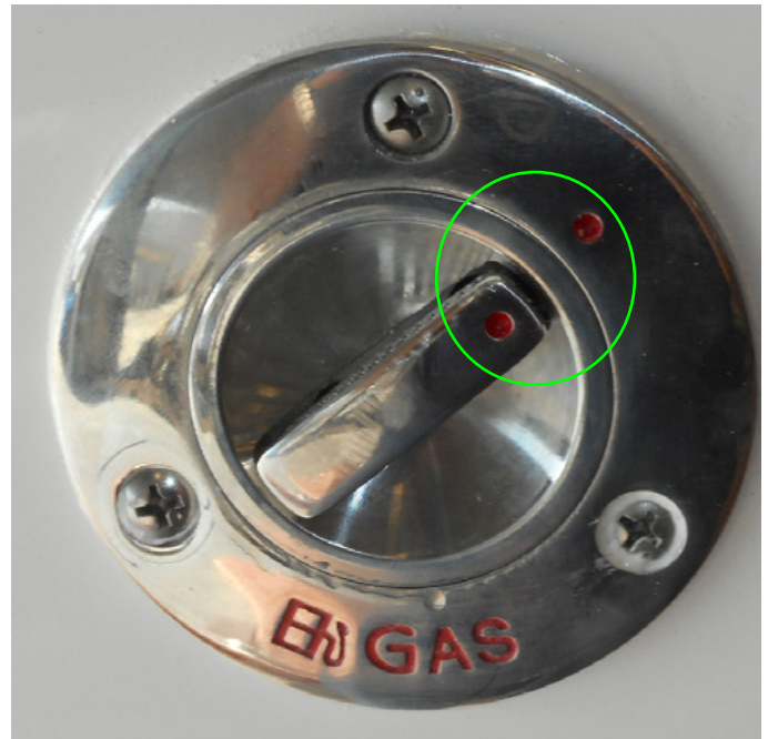
FUEL FILL CLOSED AND POINTS LINED UP
