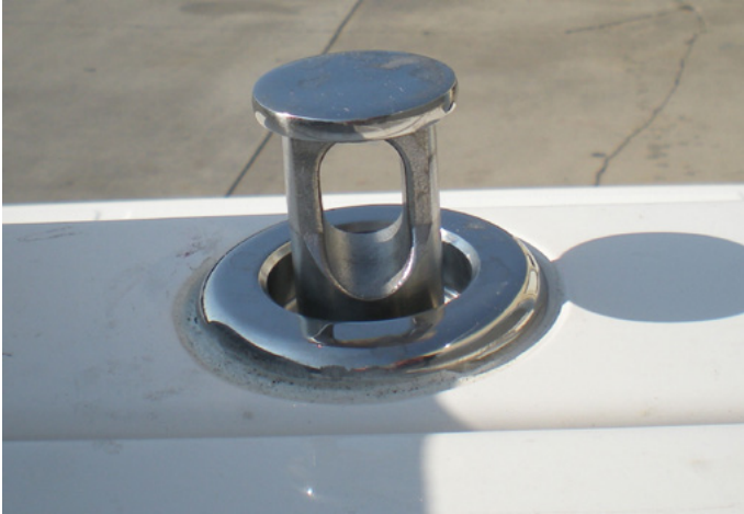
WATER SPORTS TOW DEVICE-EXTENDED POSITION
