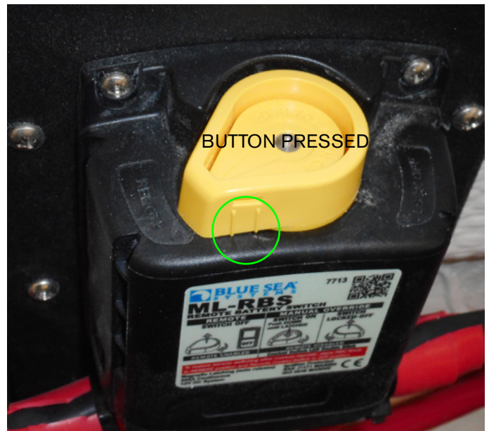
REMOTE BATTERY SWITCH- ON OR REMOTE- POSITION-(NOTE ALIGNMENT MARKS )
