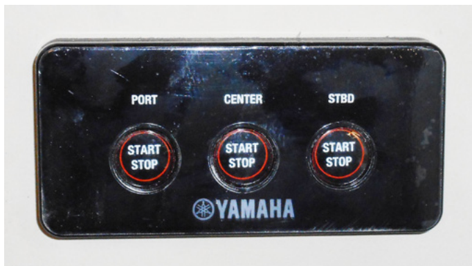
YAMAHA TRIPLE ENGINE STARTING PANEL
