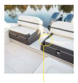
Your vessel features dual aft seats with the ability to move forward or backward up to 12" with the use of a standard switch mounted at the walk thru area. This feature permits additional cockpit space while entertaining at the dock or anchored.
