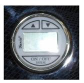
The depth gauge indicates the water depth under the keel of the boat. It features a shallow water alarm to warn the skipper of hazardous situations. By monitoring the water depth, damage to props, and underwater hardware can be avoided. This gauge is connected to a transducer on the bottom of the hull, accessible through a removable plate in the ski locker.
