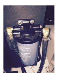
Fuel filters are installed on each outboard engine under the motor shroud (cover) which should be serviced per outboard motor manufacturer. Also, Regal installs for each outboard an in-line 10 micron water separator filter which is a spin on type similar to an automobile oil filter. Its main purpose is to trap dirt particles and condensation in fuel. It is a good idea to keep an extra fuel filter on board along with a filter wrench, catch container and clean rags for
