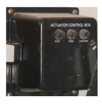
The Power Tower features an actuator control box. This component is located in the aft starboard storage compartment under the hatch area. The unit provides over current protection through a set of breakers on the face of the actuator box. Facing the box the left reset breaker protects the port power tower lift actuator. The center reset breaker protects the starboard power tower
