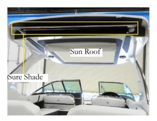
If installed, the hard top features a center soft sun roof with a built-in Sure Shade. The hard top may also include 2 speakers and a a LED accent lighting system.
