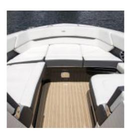
Care of the seating includes periodic cleaning with products which are non-corrosive and are recommended for vinyl. Select seats use rams and hardware which needs to be periodically checked for tightness.
