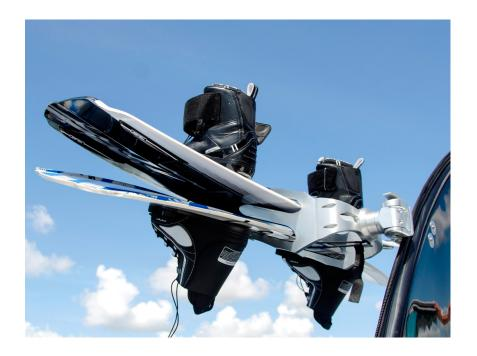
Optional board racks attach to the Power Tower. Pull up on the latch to move the board rack body. It will reach a detent and lock. Use the bungee cord to hold the boards in the slots.
