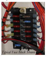
behind the dash for overcurrent of select electrical protection components. If a fuse blows determine the cause of the overload before replacig the fuse energizing the component. The fuse block shown below is a typical example of the footprint used on your vessel. Access to the fuse panels is found by removing the cover plate screws and cover plate located under the dash itself. Also, if further room is needed, the dash
