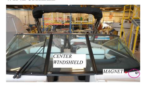
The center windshield shall be closed and locked when the boat is making headway. Make sure both locking latches are firmly seated in a horizontal position against the windshield framework. Magnets will secure the center windshield when open in a mooring or anchored environment.
