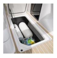
Your Regal is equipped with a floor locker which is used to store equipment such as skis, wakeboards, or larger aqua toys. To open your floor locker, pop the ring up, rotate the handle 180 degrees, and pull up on it. Your floor locker opens with the assist of a hydraulic ram. Your floor locker contains its own drain and allows access to the transducer for removal. Also, there is a special material
