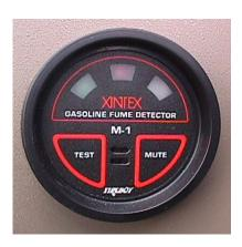
The head unit can be tested for electrical continuity by pressing the "Test" switch. The Red LED will come on. The light will glow as long as the switch is held down. If the test switch is held down longer than 10 seconds the horn will sound and the "MUTE" switch must be pushed to silence the horn.
