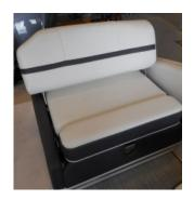
This illustration shows the seat backrest in the forward facing position. If the seat is in the lounge or aft facing position simply pull the latch and position the backrest to the rear. You will hear it as it latches in place.
