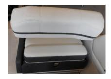
This illustration shows the seat backrest in the aft facing position. If the seat is in the lounge or forward facing position simply pull the latch and position the backrest to the rear. You will hear it as it latches in place.
