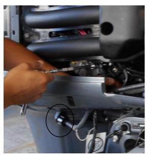
Your Yamaha outboard features a flushing device which when connected to a garden hose circulates fresh water through the engine to purge unwanted debris such as found in salty, brackish, and silty water.
