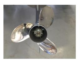
Out-of-balance or nicked propellers will effect performance or cause vibration. Damaged props should be replaced, but those that are chipped or bent can usually be reconditioned by a marine dealer or a propeller repair facility. When cruising, consider carrying a spare set
