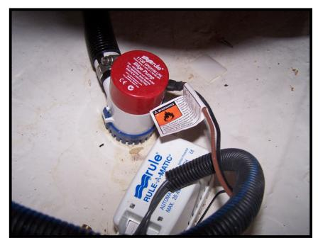
Typical Bilge Pump And Automatic Float Switch
