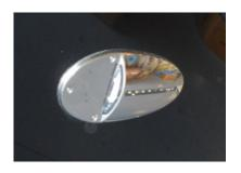
If installed, docking lights are integrated into the hull. They are very useful for night mooring approaches and maneuvering. To operate turn on the helm switch marked "docking lights".
