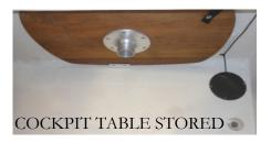
As an option, a teak cockpit table may be found in a cockpit storage locker. When using the table ensure the table pedestal leg is installed in the receiver securely. Pull the latch pin and hold until the table pedestal leg
