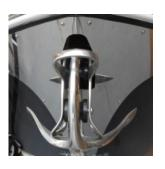
If installed the windlass features a stainless steel polished "claw" style anchor complete with swivel. This anchor has high holding power in most seabeds.
