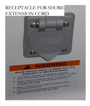
As soon as this extension cord circuit is activated it is also connected to the dock and all the other boats around you. Your boat is now part of a larger electrical system (Galvanic cell). Bottom line is that the zinc anodes on your vessel and drive may erode at a much faster rate due to stray current in the water. Zinc is more sacrificial than many other metals used on boats such as stainless steel.
