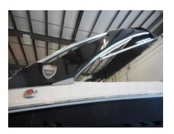
As an option the Power Tower hinges forward for tight overhead clearances such as bridges and restricted storage situations.
