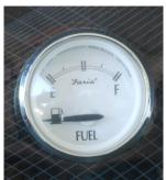
The fuel gauge indicates the level of fuel inside the fuel tank as sent by the fuel sender. It is a good idea to keep the fuel tank "topped off" when possible to reduce fuel vapors inside the tank. Do not run your fuel too low as this style gauge is not always accurate. Always allow for a "safety" factor.
