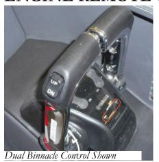
Single outboard vessels use a single binnacle control for shifting and throttle operations. The remote control handle controls forward, neutral, and reverse outboard shifting operations. Also, the control features power trim up and functions. See the following page for component description and features. Practice docking operations using the remote control in a
