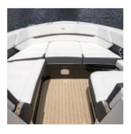
Flexiteek decking is available on selected models. It features significant advantages over similar wood products. It is made from synthetics. Color is as natural as timber and uniform through the entire thickness adding to its appeal. It sands like wood resulting in a natural wood look and feel. It provides superior grip making it great for boating in general and water sports. It is stain resistant with most
