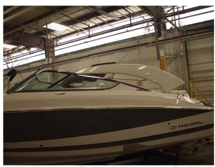
Typical Power Tower Shown In (Bridge) Full Forward Position 6-46
