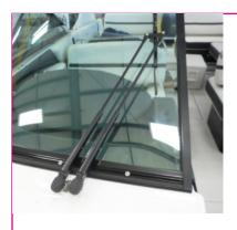
An optional driver side windshield wiper may be installed on your vessel. This wiper features a panagraphic design which keeps constant pressure on the wiper blade to ensure a more efficient removal of water on each sweep. Note that windshield damage may result if the wiper blade is run over a dry windshield. Periodically check the wiper blade for excessive wear
