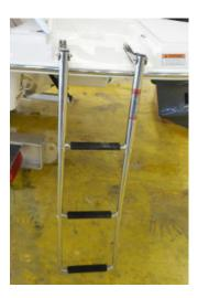
Utilize the aft swim ladder for entering and exiting the water. Use the appropriate hand rails and ladder rungs. Be sure all body parts are clear of the ladder when folding the ladder up or down. Keep body parts away from the hinged and sliding parts. Read and adhere to any written warnings posted on the dash or swim platform regarding ladder load limits.
