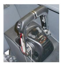
Check the helm control box and the cable attachment at the engine for tightness and shifting without binding. Shift and throttle controls at both the engine and helm areas must be checked on a periodic basis. At the engine end, make sure all control cable hardware is tight and control cable brackets are secure. An application of silicone spray on the cable ends periodically will keep control cables working freely and
