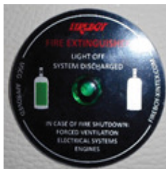
Typical Dashboard Automatic Extinguishing System Light
