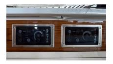
To operate your onboard grill, first make sure Live Power is on (see, "Live Power" pg. 48). Flip the grill breaker switch, under the port side mezzanine seat, on. There are two grill control panels in the center of the refreshment island on the forward face. Press the "ON/OFF" button on each control panel to turn the grills on and then press the unlock button to unlock the grills. Use the 'plus' and 'minus' buttons to control the grill's temperature.
