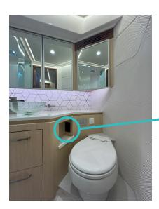
Reset the GFCI from the outlet in the head or the outlet behind the V-berth seating. When tripped, the top button on the outlet will pop out. Press it in until it clicks to reset the breaker.
