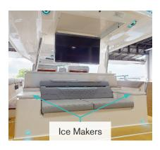
Tap the snowflake icon on the DSS to turn the ice maker. The ice maker will turn off when ice level reaches a shut off sensor in the bin.
