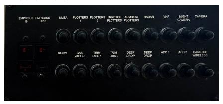
The "12 Volt Helm Panel" breakers helm electrical components including the plotters, VHF radio, and trim tabs.
