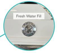
Unscrew the cap, thread one end of your freshwater hose to the water source and the other into the fill valve. Freshwater hoses are normally white, can be purchased from any home improvement or marine supply store, and do not leave a rubbery taste in your drinking water. Turn the water source on and fill the tank until the freshwater icon in the DSS reads full. Turn the water off, disconnect the hose, and replace the valve cap.
