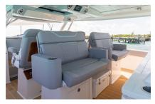
There are two rows of cockpit seating on the 50 SAV-a row of four helm cockpit seats, equipped with foldable armrests, and a pair of sleigh seats behind them. The sleigh and outer helm seats rotate 180°. To rotate the sleigh seats, tap the seat icon on the "Deck" page in the DSS. A window will pop up. Hold the curved arrows to rotate the sleigh seats. Do not sit on the seat while rotating.
