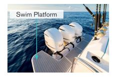
Make periodic inspections of all hardware that supports the platform including the ladder. Ensure that all connections and fittings are tight and in good condition. Always retract the ladder and secure in the locked position before making headway.
