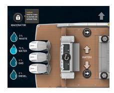
The droplet icons along the left side display the gas, diesel, waste, and freshwater levels. Tap the waste icon to enable the macerator. Hold the macerator icon to activate the pump.
