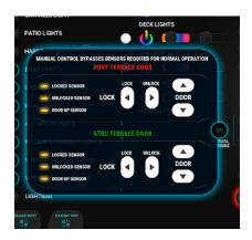
When the lock is fully retracted, press and hold the down "DOOR" arrow. Attempting to lower the door while the lock is engaged will damage the vessel.
