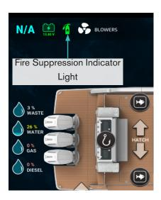
There is a "Fire Suppression" indicator light within the DSS (see, "Digital Switching System pg. 63). When the system is charged and ready to detect a fire, the light will be green. If the system has detected a fire and is discharged, the light will flash red and an alert message will display on the Garmin plotters.
