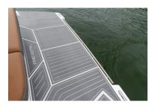
Your vessel may be equipped with optional Seadek or ReFlex matting. Matting is made of UV protected, non-absorbent foam that stays cool to the touch and maintains traction even when wet. Upgraded matting is designed to resist stains and, most of the time, hosing down the matting is enough to keep it clean. If more thorough cleaning is required, use any, non-acid based household cleaners and soft rags or soft bristle brushes to remove any dirt or residue.
