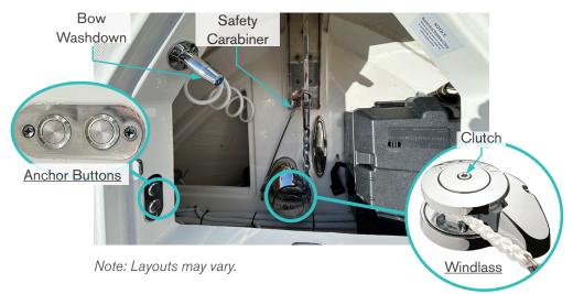
You can control the motor with the buttons inside the anchor locker or on any plotter via the DSS (see, "Digital Switching System" pg. 63).
