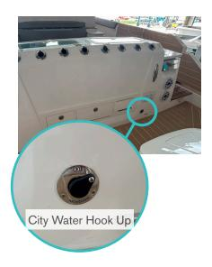
Your freshwater system can also run from an onshore water source when docked. To connect your boat to an onshore source, remove the cap from the city water valve on the aft face of the fishing tombstone toward the lower starboard side, below the shore power compartment.
