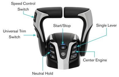
Your boat comes equipped with a twin control Yamaha EX Shifter. The left lever controls the two port engines and the right lever controls two starboard engines. Press the "Single Lever" button to control all engines together.
