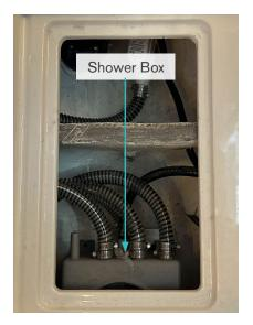
A gulper pump on the starboard side of the engine compartment pumps water out of the shower box and overboard through a thru hull fitting on the starboard transom. Check the pump periodically for debris blocking the pump grate.
