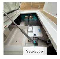
Turn the Seakeeper breaker on at the MDP and verify that the seakeeper handle on the water manifold is horizontal (open) before operating (see below).
