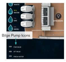
Your bilge pumps operate both automatically and manually. Float switches will automatically activate a pump when necessary. You can manually activate the bilge pumps from the DSS. Icons in the DSS will also indicate when a pump is active, whether triggered automatically or manually (see, "Digital Switching System" pg. 63).
