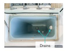
Water will continuously overflow through a cutout in the lid gasket at the outboard aft corner of the lid. The overflowing water will run down the aft side of the tombstone and onto the swim platform. Adjusting the top drain changes the amount of water that overflows the gasket. Twist the drain to adjust.
