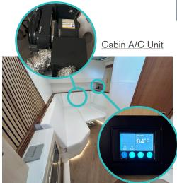
The raw water loop through the A/C units returns to the Lazarette where it discharges through a thru hull in the transom. The unit comes equipped with a sound cover and dedicated vibration isolation system that will help reduce noise.
