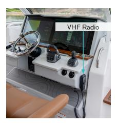
Very high frequency or VHF radios are used for distress signaling, ship to ship, and ship to shore communication. All Regal boats leave the manufacturer with a VHF-FM radio installed. Channel 16 is the primary channel for ships in distress.
