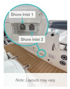
Connecting to shore power will automatically begin charging the Power Bank. If any AC equipment is on while connected to shore power, the Live Power system will power the equipment while the shore power charges the Power Bank. If too many devices are on while charging, the onshore source will power equipment instead of charging the Power Bank. Connecting to shore power will disable the auto-generator feature.
