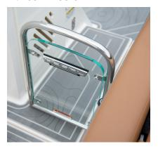
The transom doors separate the stern seating area from the swim platform. To open, lift up on the door and swing the door forward. To close the doors, lift up on the door and release once the door is in place. Keep both transom doors closed while underway to avoid injuries or damage to the vessel.
