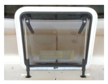
Most deck hatches feature a locked position. To lock the hatch first grab the handle and turn it so it engages the side of the seal ring as shown. Push the lock mechanism to engage the handle in the locked position.
