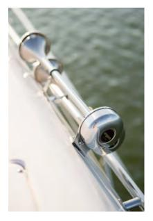
The typical air horn set features an air pump which is located under the salon whisper wall ceiling covering. The horns emit a sound that can be heard much louder than the typical electrical horn. This extra distance capability can be useful in ship to ship crossings especially when foul weather is present.
