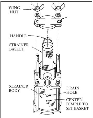
Before servicing the sea water strainer make sure the appropriate seacock has been closed to prevent water entering the boat. If possible blow out the strainer basket with compressed air or use a metal type brush to remove any accumulated material from the screening material. Make sure the strainer is aligned in the center dimple on reinstallation.
