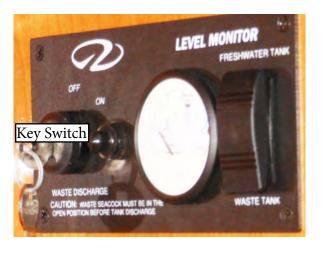
FRESH WATER & WASTE MONITOR WITH OVERBOARD DISCHARGE
