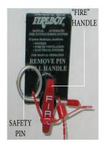
If a fire has started in the engine compartment find the system manual cable assembly located in the cockpit. Remove the safety pin from the "Fire T Handle" and pull firmly on the "Fire" handle which will activate the fire extinguisher unit in the engine compartment. A loud "rushing air" sound may be heard. Complete discharge will take several seconds. Keep the compartment closed for a
