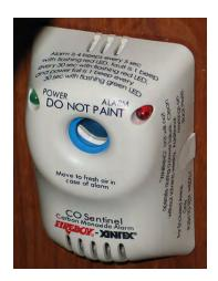
3. The test cycle should be activated frequently. Simply press the button. When it is released, the (top) power indicator will flash off and the lower indicator light will flash on. Then, the lower indicator will flash off and the upper indicator light will come back on.
