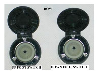
On select models bow foot switches are used to control the windlass. To use the foot switches remove the protective caps. When you energize the up foot switch the anchor is retrieved. When you energize the down foot switch the anchor is payed out. After the anchoring process is completed close the protective caps.
