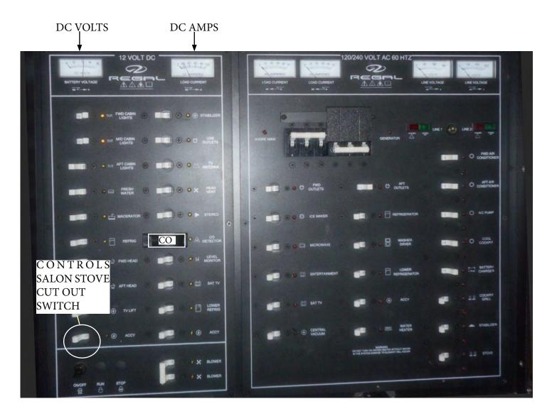
The main DC control panel is located near the salon stairway behind a set of cabinet doors. The port panel protects direct current circuits. The starboard panel protects AC circuits. This panel is protected by the cabin main breaker at the battery management center. The panel features an analog 12 volt DC volt meter and amp meter to monitor electrical flow and current. These 2 instruments can be valuable aids in basic electrical troubleshooting.
