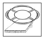
TYPE IV- Intended for calm, inland water with heavy vessel traffic, where help is constantly present. It is designed to be thrown into the water for someone to grab on to and held until rescued. It is not designed to be worn. Type IV includes ring
