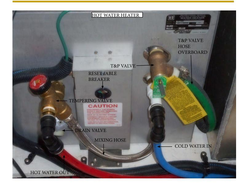
The hot water heater features recirculating ability to keep water warm during cruising. This is accomplished by a set of hoses connected between the hot water tank and the circulating engine water pump.
