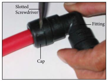
2. Push the connector and collar together. Hold the collar next to the connector with your finger. Pull and the connector/collar will release itself from the water line.
