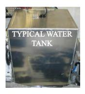
Your vessel is equipped with a fresh water supply referred to as a potable water system. It consists of fresh water tanks, dockside fill/vent fittings, monitor panel, pressure water pump with filter, distribution lines, manifolds, wash down spigots and hot water heater.
