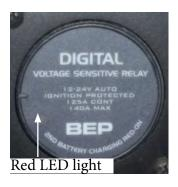
Located on the battery management panel are 2 VSR's (voltage sensitive relays). The purpose of the VSR is to protect the engine batteries from being discharged. Also, when the engine batteries are fully charged it sends current to charge the house battery.
