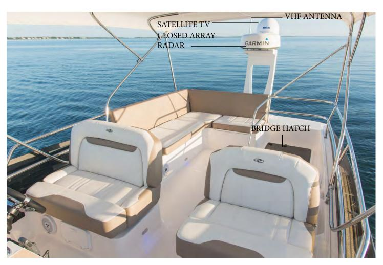
The photo above displays a typical bridge layout. Note the electronics mast which may feature closed array radar along with satellite television domes. Also, a VHF antenna is found here.
