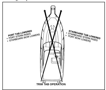
Using trim tabs will compensate for uneven weight distribution, listing, water conditions, wind velocity and other factors that cause inefficient operation.
