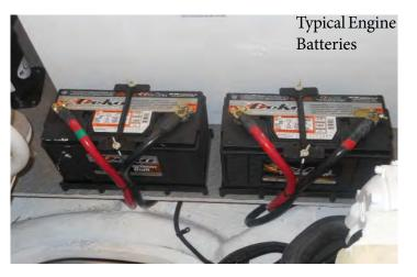
Tighten all battery connectors securely. Check their tightness by pulling on the connectors. They should not move from their tightened position. Be sure to reinstall the positive boot over the battery terminal after tightening the battery post connection. While using the boat, keep an eye on the volt meters to monitor the charge level of each battery bank. Monitor the charge with the engines turned off (static condition).
