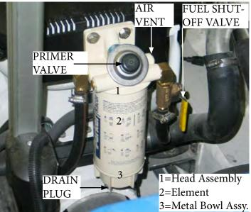
RACOR WATER SEPARATOR DIESEL FILTER
