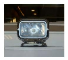
The spotlight feature a 20,000 candle power light beam which can penetrate up to over 1/2 a mile in ideal conditions. The 2 speed searchlight provides up to 370° horizontal rotation and up to 135° vertical tilt with a dash
