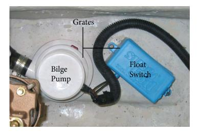
Your vessel offers as standard equipment a bilge pump service. Periodically check the grates for debris and test spray the units down with water. Make sure that a steady stream of water exits the through hull fitting indicating the hose from the bilge pump itself is clear. Periodically check all hoses, clamps and electrical con-
