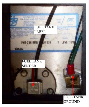
Placed at the top of the fuel tank is an electronic fuel sender. This device reads the amount of fuel remaining in the fuel tank and sends a signal to various displays including the fuel system display on the Garmin chart plotter(s)..
