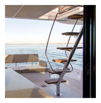
The bridge entry way stairway features wide treads and a handrail system to provide safe access to and from the bridge. The teak steps can be maintained by periodically using teak reconditioning products. Be sure to wipe treads off sufficiently to remove any residue .Use a stainless steel polish as needed to retain the corrosion properties of the hand rails, etc.
