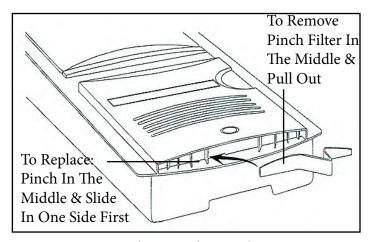
Replacing Exhaust Filter
