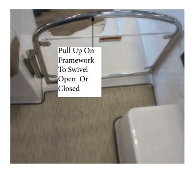
To open the door (gate style) pull <u>up</u> on the framework until the door hinge releases and swivels to an open detente position.
