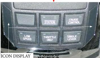
Station button- featured for multi-station boats. Since Regal yachts feature one helm the station button lights up "green" when the control is activated but this function can't be configured.
