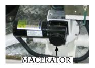
The macerator (overboard discharge pump) option is located in the engine room. It is connected to a normally closed seacock. In locals where it is approved the seacock is opened and
