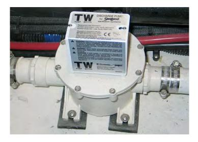
If your boat is equipped with an overboard discharge pump pay close attention to what materials are flushed through the waste system as it could become clogged. Do not pump garbage, rags, or sanitary napkins through the overboard discharge pump (macerator). Flush the waste tank and pump with fresh water with each pump out. Do not run the pump dry or for extended periods of time since the impeller can be damaged.
