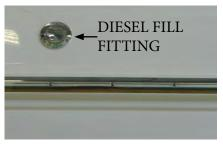
Fuel tank fill fittings are normally located on the deck. They are marked diesel. Never pump gasoline in a fuel tank designated for diesel fuel. After
