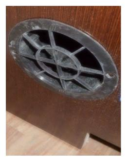
Note that to the port and starboard lower sides of the berth are found air conditioner takes for the forward air conditioner These unit. grates mix air and are part of the return air system.
