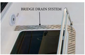
The bridge drain system evacuates runoff bridge water and sends it overboard via a hull side fitting. The stainless steel cover can be removed as needed to clean any debris in the drain holes or the drain raceway.
