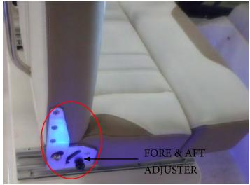
The bridge helm seat is adjustable fore and aft through a lever rod component located under the front of the seat. Simply push the rod to the right and while holding it in position push the seat back to the desired location and then release the rod. it will lock the seat in the nearest track detent.
