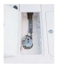
The typical windlass needs periodic maintenance to keep it in top running condition. Every 6 months the manufacturer recommends that the unit be disassembled and all the above deck parts be washed down with fresh water. Lightly oil (SAE 10) the seal, shaft, cone clutch and spline. Ensure that the
