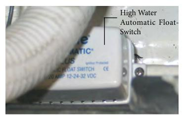
The high-water alarm warns the skipper of a possible emergency in the bilge area. There is an automatic float switch installed in the bilge. If the water rises over a predetermined level the bilge float switch sends a signal to the helm mounted alarm. This sump float switch normally is elevated from the position of the automatic 6. Seacock leak. bilge pump switches.
