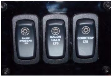
To use the dimmer switches depress the desired switch for on and off. The lights will appear at their brightest mode. If you want to dim a particular switch circuit simply depress the lower portion of the switch and hold the switch in that position. The lights will dim until you release the switch.
