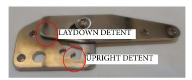
Note the position of the seat hinge. To travel from the upright to the lay down position pull up on the seat to engage the seat in the lay down detent section of the hinge.
