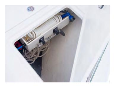
Under the forward deck locker is a wash down hose and faucet. To use make sure the fresh water breaker is energized on the ship's main DC panel, turn on the faucet, pull the hose assembly out of the storage cavity and adjust the hose nozzle to the needed spray pattern.
