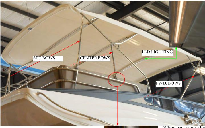
The bridge features a bimini top which affords shade from the sun and protection from the elements. It is a light, UV protected marine fabric. The top assembly is furnished with a complete set of stainless steel bows for durability. The top utilizes 3 sets of bows to assemble or disassemble the cover.
