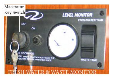
To read either the fresh water or waste water monitor panel the breaker on the main DC panel must be activated.
