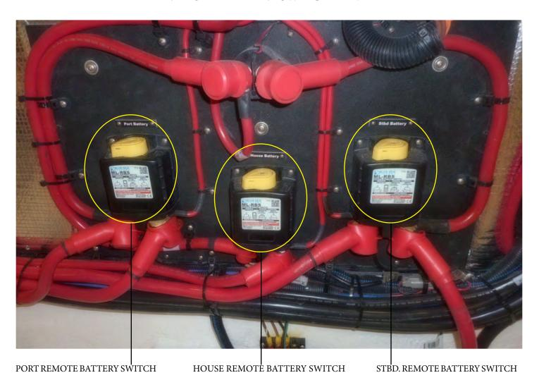
As part of the battery management system 3 remote battery switches are located in the engine room.
