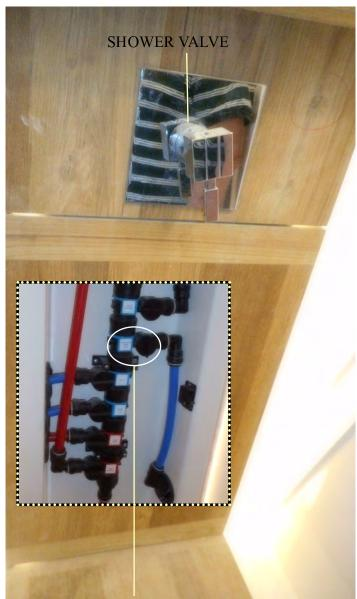
MASTER SHOWER TEAK LOCKER- FRESH WATER SYSTEM TANK SHUT-OFF VALVE INSIDE
