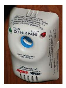
Use the following procedure monthly or when leaving the vessel for extended periods. Normal maintenance should include frequent checking for the green power light glowing with the warning indicator and audible horn off. The detector should b e
