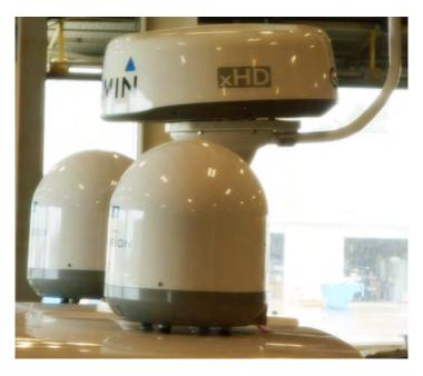
If installed, the satellite television option typically features the ability to viewing hundreds of television channels using the salon TV. Basically, the signal is transmitted through an antenna system installed on the hardtop which features a satellite tracking system that automatically finds the satellite for crystal-clear television reception. To activate satellite television a subscription must be secured. For more information call 1-800-970-9623
