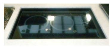
The salon galley mounted stove features 240 volt power and a ceramic cleaning surface. There is a safety switch back up system integrated into the wiring circuit. The unit offers 2 large size burners and a variety os temperature settings.
