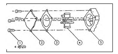
The oil changer system requires little maintenance up to the 500 hour period. At that time the impeller needs to be replaced. Earlier replacement may be necessary if the oil changer has been operated dry, foreign objects have broken the impeller vanes down, or improper liquids have been run through the system. For impellers and gaskets, call 1-800-922-4804.
