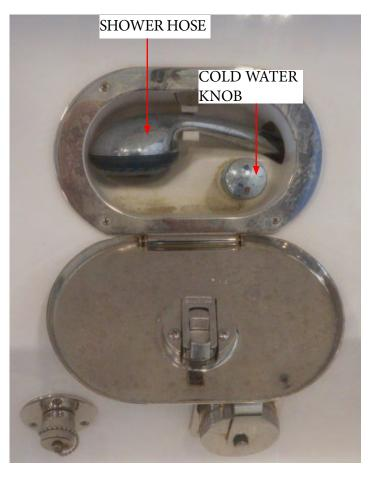
If installed the transom shower is located at the starboard transom. It features a cold water sprayer with sufficient hose to rinse passengers entering from the water, etc.
