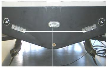
Typical Ocean Trac Bottom Using Shims Around Anodes
