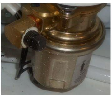
TYPICAL GENERATOR INTEGRATED FUEL FILTER
