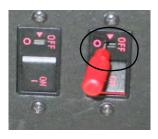
A. Take a small slotted screwdriver from your on-board tool kit and insert it in the breaker slot until it trips. You will hear a snapping type noise. See the illustration.
