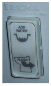
The wall control switch is used to add water to the bowl and to flush the toilet. Select cycle information is noted below. For more complete information, refer to the toilet vendor information located in the information packet.
