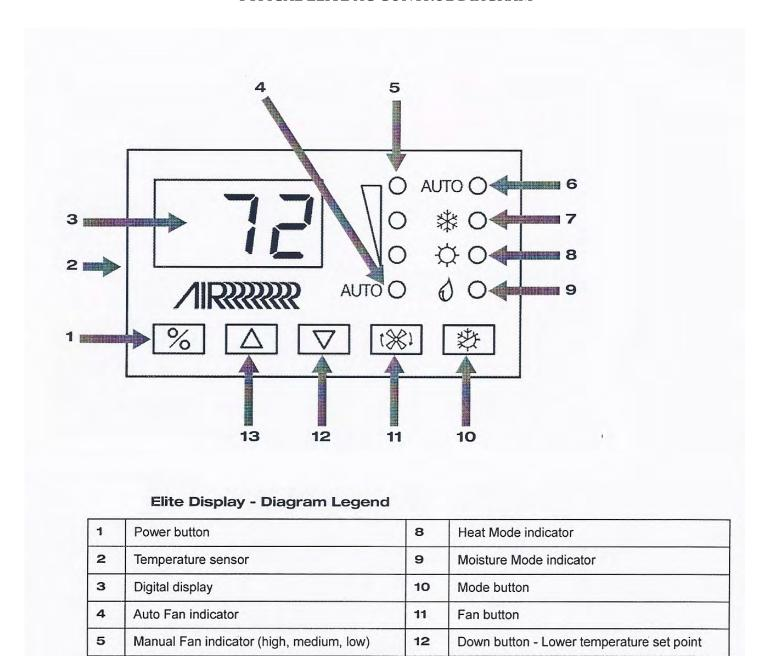
Note: The Elite display continually monitors the system components. Should a problem develop it sends a diagnostic code to the control (thermostaat) display. Refer to the vendor air conditioning manual (troubleshooting) to assist in identifying the problem.
