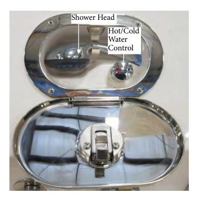
The transom shower is located at the starboard transom area. The shower head features a flexible extended hose with a hot/cold water control knob. Like residential plumbing, the red dot denotes hot water and the blue dot cold water. When using this feature balance the hot and cold as required to achieve a desired and safe operating temperature. Turn the control knob to the "off" position when not using the unit.
