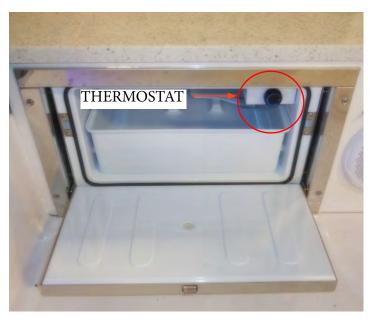
It fits under the bench seat. It features a pull-out tray to for easy access. At the upper right of the unit notice the thermostat control. Turn the knob clockwise to make the temperature cooler or counterclockwise to make temperature warmer.
