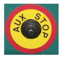
To stop the engine should the key fob system fail to shut down the engine there is an auxiliary stop switch located in the sump on the side of each engine. Depress the button until the engine completely stops. See the illustration.
