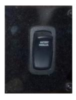
The battery parallel switch is connected through the engine ignition switches to each of the engine cranking batteries. If one of the engine cranking batteries is weak this system will use the good battery from the one engine to provide cranking power for the weak battery of the other engine.
