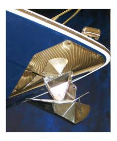
Your Regal yacht features a stainless steel plow type anchor. The anchor will set quickly in a variety of bottoms because of its unique shank profile and ballasted tip. It is a high holding type anchor made from high grade manganese steel and stainless steel
