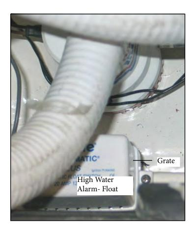
The high water alarm float is located in the engine room. Periodic maintenance consists of visually inspecting the float grate cover for debris and removing any accumulation.
