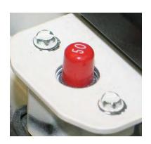
The IPS drive unit 50 amp breaker is mounted near the top of the engine close to the dual oil filters. It protects the drive unit from being overloaded. If a breaker "pops" always figure out the reason why before resetting or replacing it. Also, there is a 20 amp
