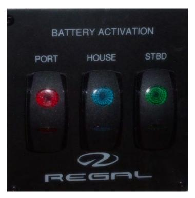
Note that when the battery switches are activated they will generate a light which alerts the skipper. Red for port cranking battery, blue for house battery, and green for starboard cranking battery.
