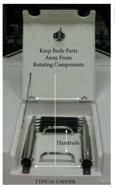
Insist that only one person use the ladder at a time. Periodically check the ladder hardware for tightness and corrosion. Replace fasteners and lubricate hinges as needed.
