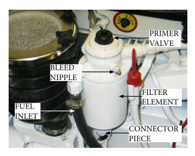
To Drain, Prime Or Replace Secondary Fuel Filter Element
