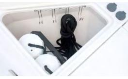
Fenders are normally made of a rubberized plastic and are usually filled with air. Most have a fitting like a
