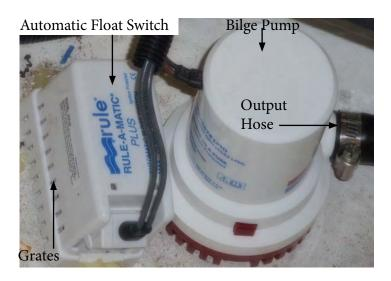
Your Regal yacht features bilge pumps and float switches in the sump (bilge) and forward cabin (selected models). They are operated through the helm switches. There are separate switches marked forward and aft bilge pumps. In the "off" position both switches are connected into the automatic float switch. In this "auto" position if the boat takes on water, the bilge pumps will activate and pump excess water overboard. The switch will light up when activated.
