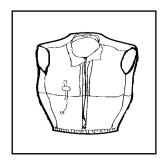
TYPE V- Also known as a special use device this is the least bulky of all PFD's. It contains a small amount of inherent buoyancy, and an inflatable chamber. It is rated even to a Type I, II, or III PFD (as noted on the jacket label) when inflated. Some Type V
