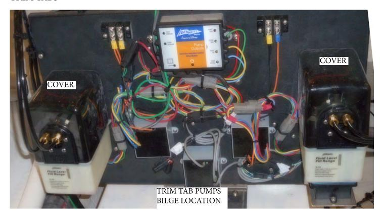
Trim tabs are located on the outer edges of your yacht transom below the swim platform. All mechanical and electrical connections should be periodically checked for tightness, corrosion, and chafing. If a malfunctioning tab is suspected, run each tab in and out while someone looks at each tab to make sure it is moving up and down the proper distance. Replace any zinc anodes mounted on trib tabs when at one half their life as determined by size. Check anodes twice a month.
