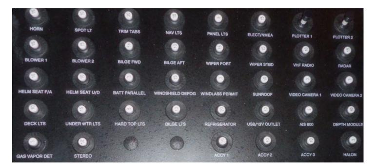
The helm breaker sub-panel protects various components located in the vicinity of the helm area. The sub-panel is controlled in part by the <u>dash main breaker</u> and the <u>electronics breaker</u> both located on the battery management center panel.
