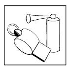
According to both Inland and International Rules, all boats must carry a way of producing an efficient sound signal. If your vessel is 12 meters (39' 4") or longer, a power whistle or power horn and bell must be carried. Bell mouth must be at least 7 7/8"
