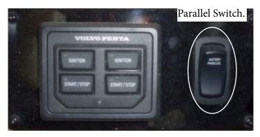
Your vessel uses the Volvo E-key system. It features a dual E-key panel with ignition and start-stop switches along with s sensor to unlock the system when a key fob is swiped at the panel.
