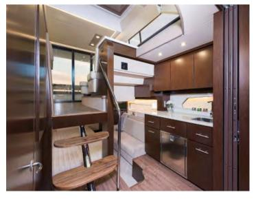
The handcrafted interior cabinets feature a sprayed clear coat finish. This clear coat produces a hard finish which is baked on and is very resilient. Use a warm solution of water and mild detergent to keep the cabinet surfaces looking new. Wipe the surface with the solution using a soft damp cloth, and dry with a soft clean towel. This procedure should eliminate most stains and oily finger marks.
