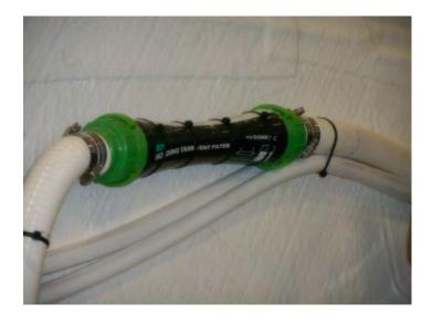
There is a waste filter installed in the vent line between the waste tank and a thru-hull fitting. The filter's purpose is to keep objectionable odors to a minimum from the waste tank. It is recommended that the filter be changed yearly. It can be ordered from your Regal yacht dealer or from marine supply stores. Typically the waste filter is mounted in the sump (engine compartment). Note that the filter exits through a transom fitting near the starboard swim platform area.
