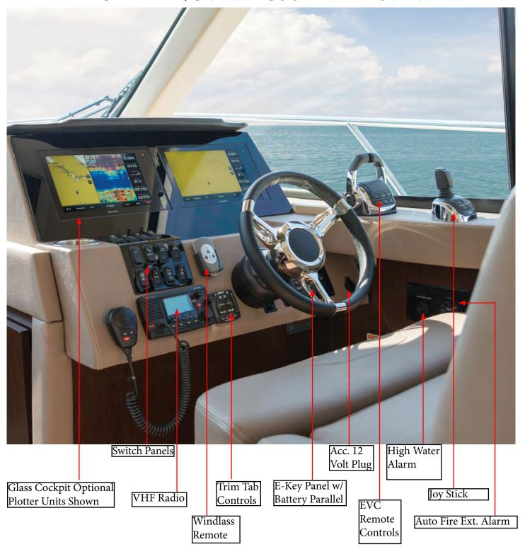
Note: Various components above are optional equipment. Location and components shown may change at any time.
