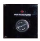
Using a bilge float sensor this component determines a high water bilge situation and sends a signal to the dash alarm. This may indicate that a large amount of water has entered the hull or there is a leak in the engine water circulation system
