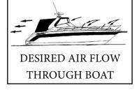
To help prevent carbon monoxide accumulation, ventilate your cabin and cockpit while underway. Open a forward hatch, porthole or window to allow air to travel through the boat's interior and
