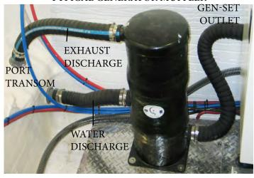
Before departure always check the hose connections for signs of water and air leaks. Tighten hose clamps as needed.
