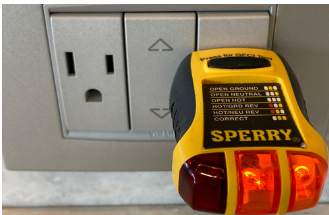
TESTING GFCI DOWNSTREAM OUTLET
