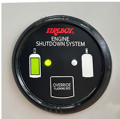
Fireboy shutdown panel
