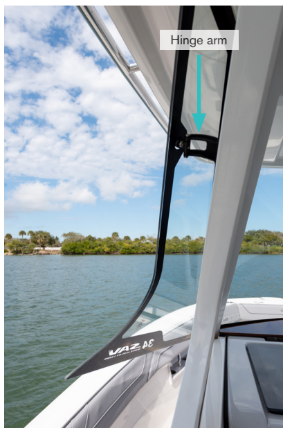
Wind deflectors deployed
