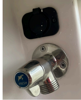
Starboard freshwater washdown tap
