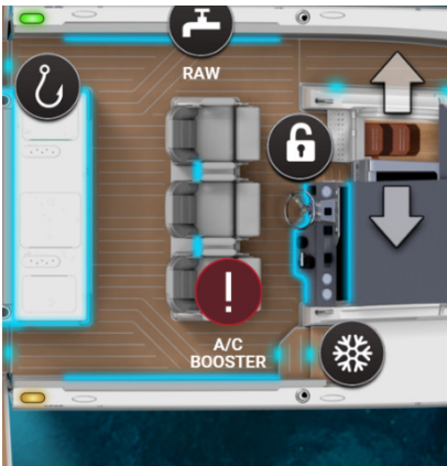
Tripped digital breaker example
