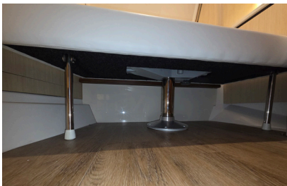
Filler cushion installed
