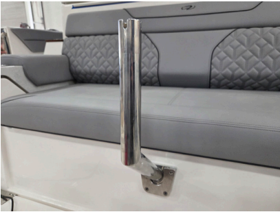
Support post installed
