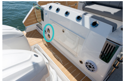
Shore power inlets
