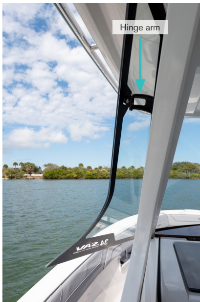
Wind deflectors deployed
