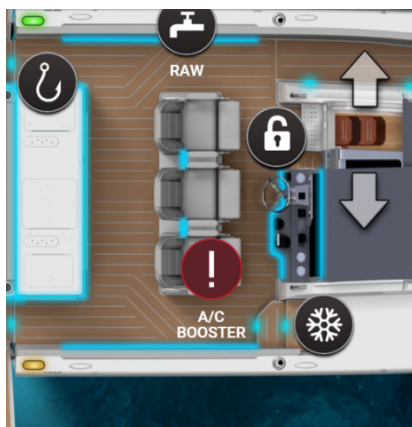
Tripped digital breaker example
