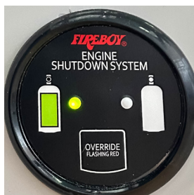
Helm shutdown panel
